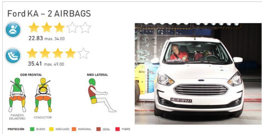
Figure 8. Ford Ka test result
