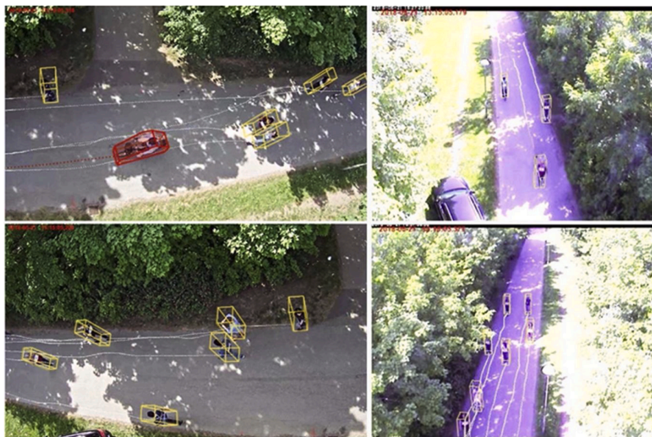
Fig. 3. A screenshot of the T-Analyst software (E-bike and pedestrians inside red and yellow boxes respectively).
