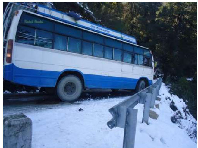
Figure 4.4: Roadside Barriers in Nepal. The GRSF funded construction of roadside barriers on cliff-side roads in Nepal, showing in order the road without barriers, during construction, at completion, as well as an example of a bus which was prevented from going over the cliff by the barrier
