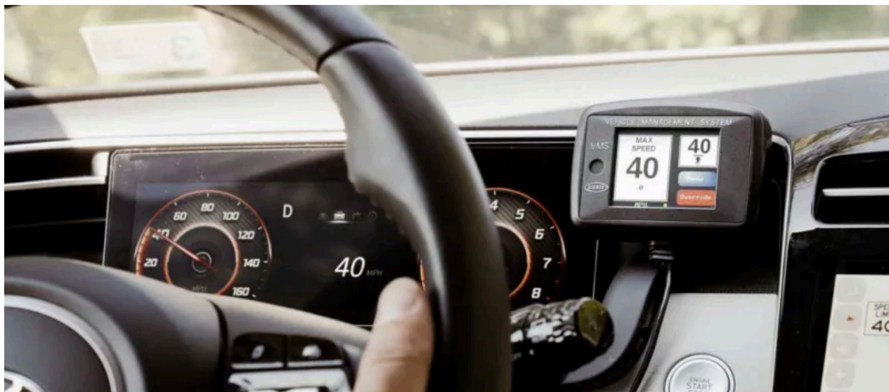
Intelligent Speed Assistance (ISA) devices can deter dangerously high speeding, particularly useful for repeat Super-Speeders. Source: IIHS
