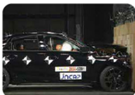
Full frontal collision test
