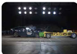
New offset (MPDB) frontal collision test
