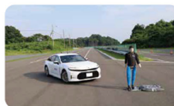
AEBS intersection : car to pedestrian (right / left turning-crossing)
